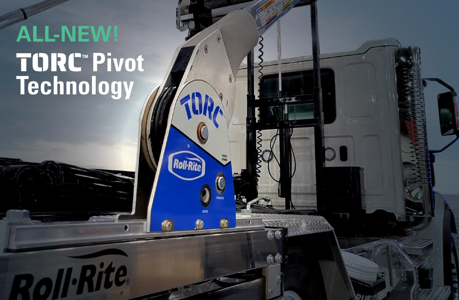
The industry's first Tension Operated Rotary Cam pivot technology with NO steel springs or hydraulics.
