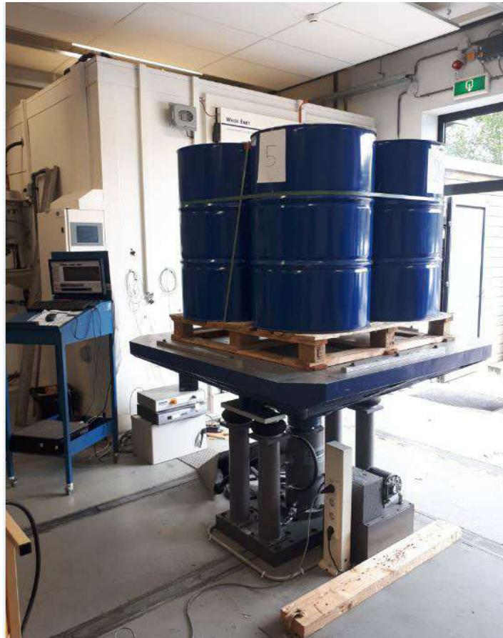
Figure 6. Test setup for vibration test
