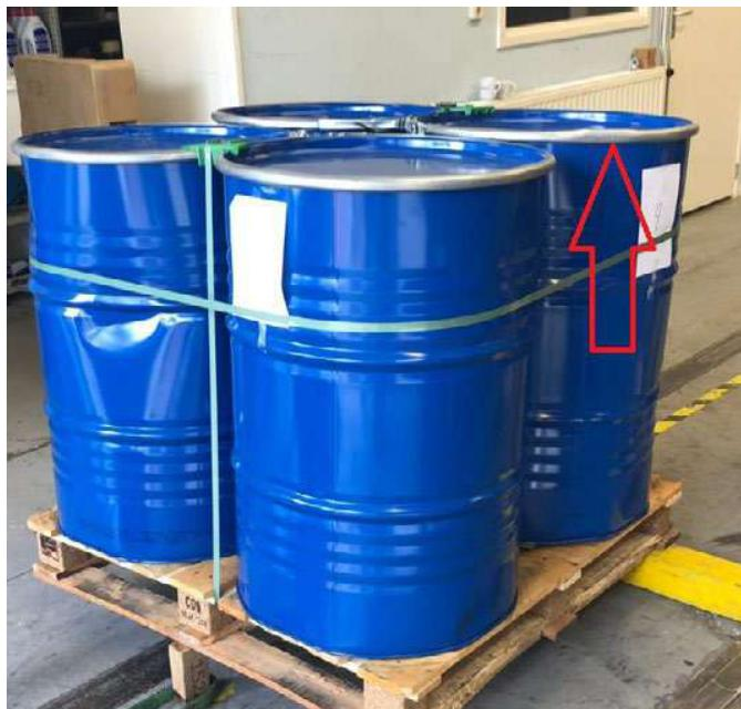
Figure 8. Damage to drum ring; only face 4.
