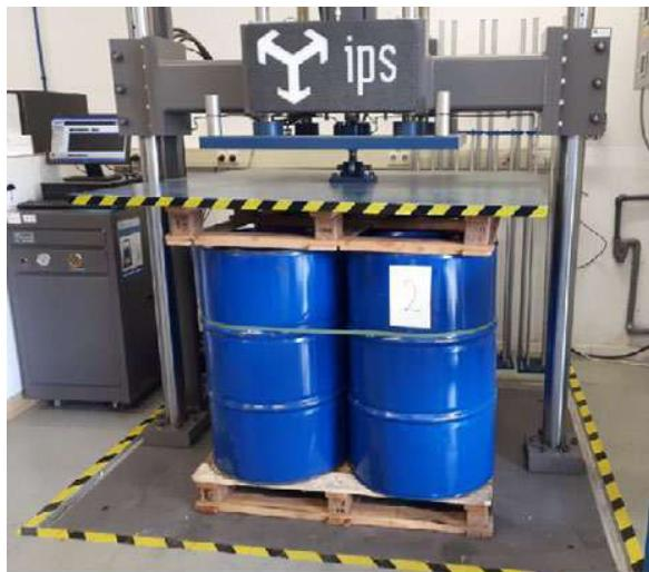
Figure 5. Test set-up Compression Test
