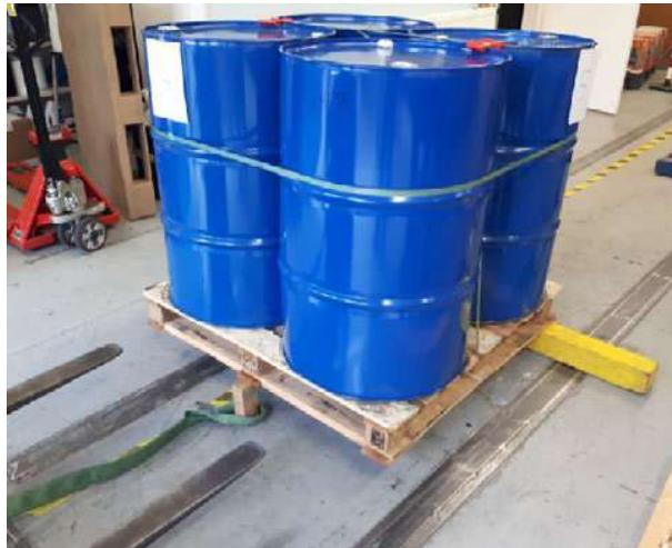
Figure 7. Set-up Rotational Edge Drop Test
