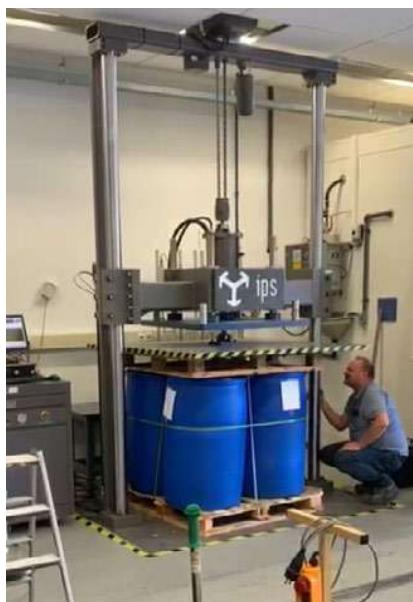
Figure 5. Set-up compression test
