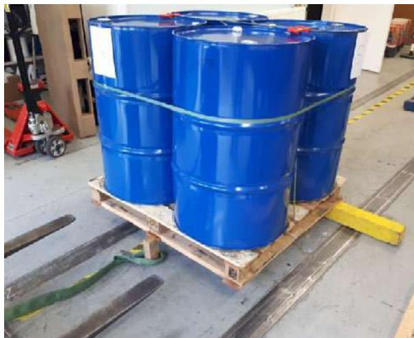
Figure 4. Set-up Rotational Edge Drop Test
