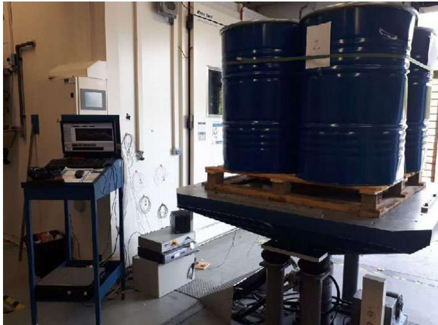
Figure 6. Test setup for vibration test
