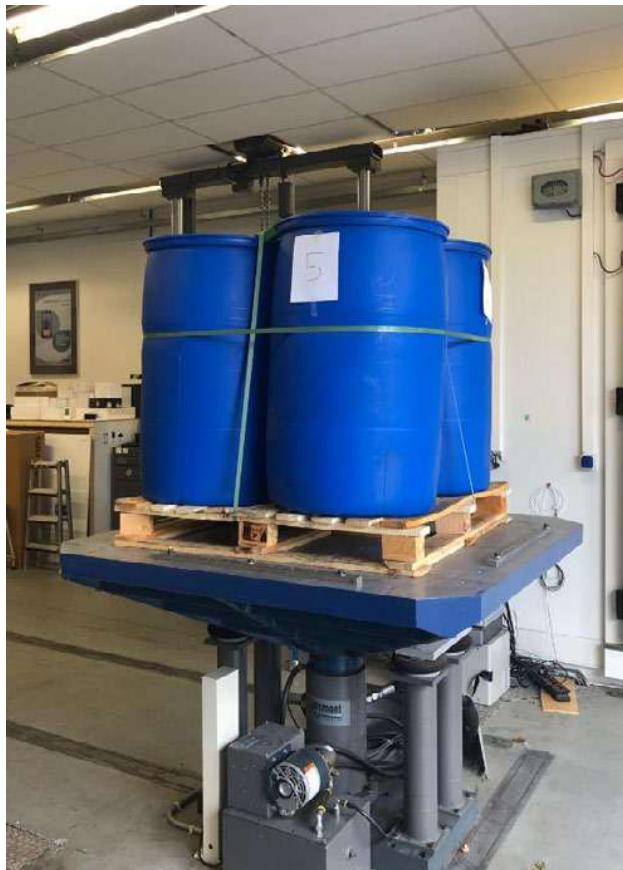
Figure 6. Test setup for vibration test
