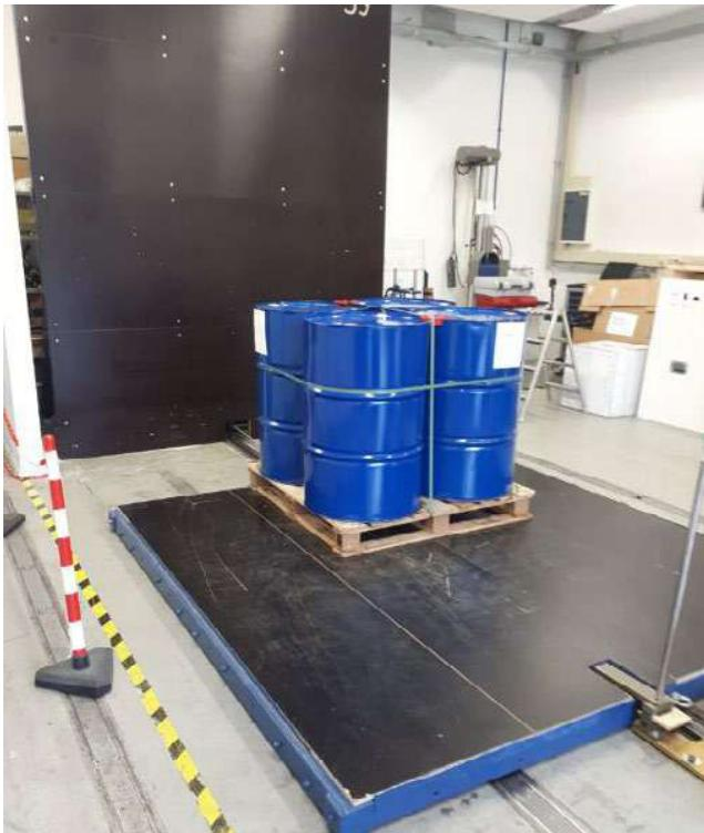
Figure 3.DUT on horizontal impact tester.
