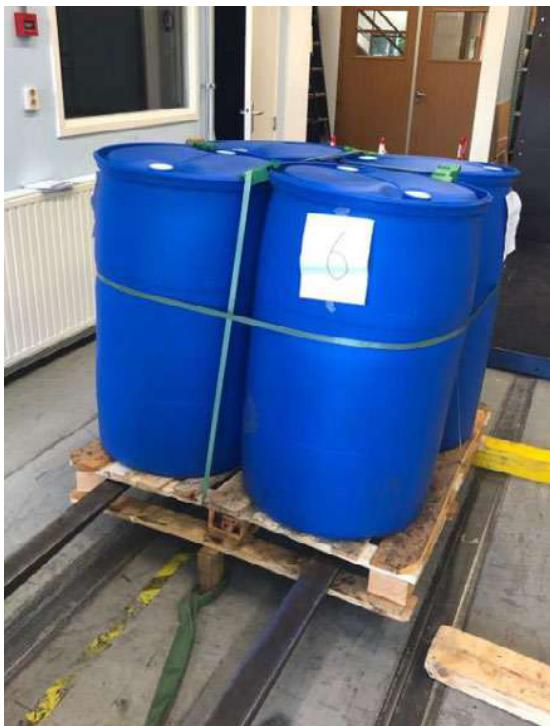
Figure 4. Set-up Rotational Edge Drop Test
