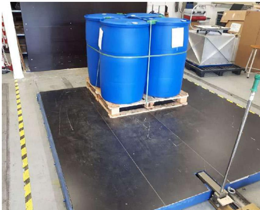
Figure 3.DUT on horizontal impact tester.
