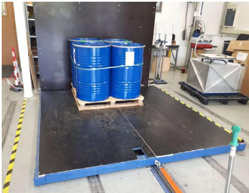
Figure 3.DUT on horizontal impact tester.
