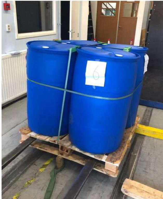
Figure 7. Set-up Rotational Edge Drop Test
