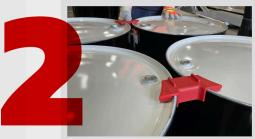
Place 2 Drumclips on the outside of the drums
