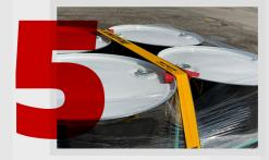
Secure the pallet to the trailer using tension strap
